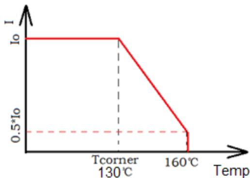
**Fig. 3 Temperature compensation curve**
